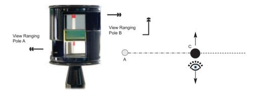
Take up a position roughly in line between Poles A and B. Look through the window and sight pole A in the lower window and pole B in the upper. Move forwards or backwards at right angles to the line until the two poles appear to coincide. The Optical Square is now in line between A & B and point C can be marked.
