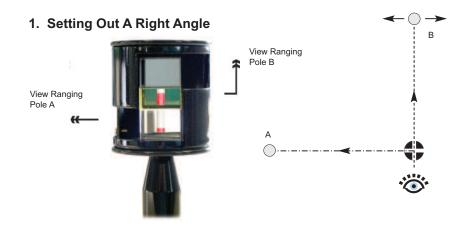
Hold the Optical Square over the alignment point, using either a plumb-bob or ranging pole to centre. Sight to Ranging Pole A through the lower prism. As Ranging Pole B is moved, view it through the centre window until the two images appear to coincide. The angle A to B is now 90° at the alignment point.
